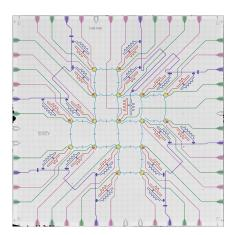
a single device. Nine physical qubits are used to encode the quantum information in an error-protected logical qubit. Eight qubits are used to detect the occurrence of two types of errors in the system: bit-flip errors and phase-flip errors, where the latter occur only in quantum computers and the former occur both in conventional and quantum computers. The <u>device was designed at ETH Zurich</u> by
