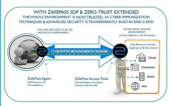
The above figure represents a simplified layout of ZafePass Virtual Private Connectivity solution. The Access Point can easily be placed in AWS, Azure, Google, Alibaba, IBM cloud environments—or at a local cloud service provider.
