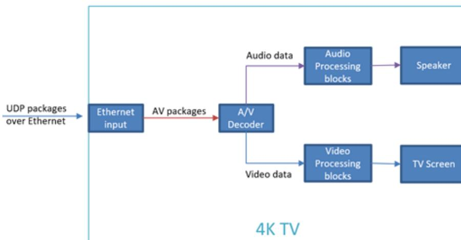
**Figure 6-72 Basic diagram of Linux based 4K TV application**
