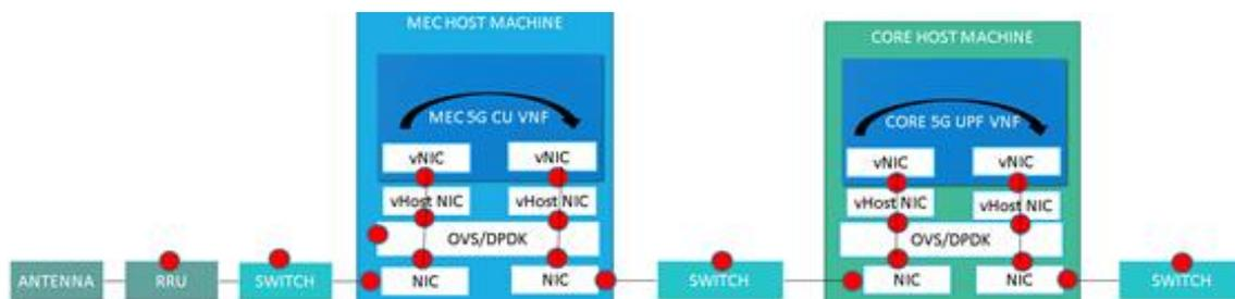
**Figure 4-53 Hybrid data plane network slicing**
