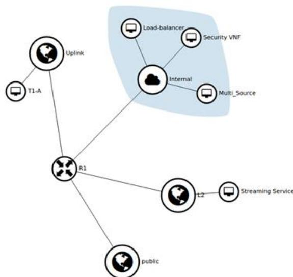
**Figure 4-43** snapshot of the network topology at the OpenStack dashboard
