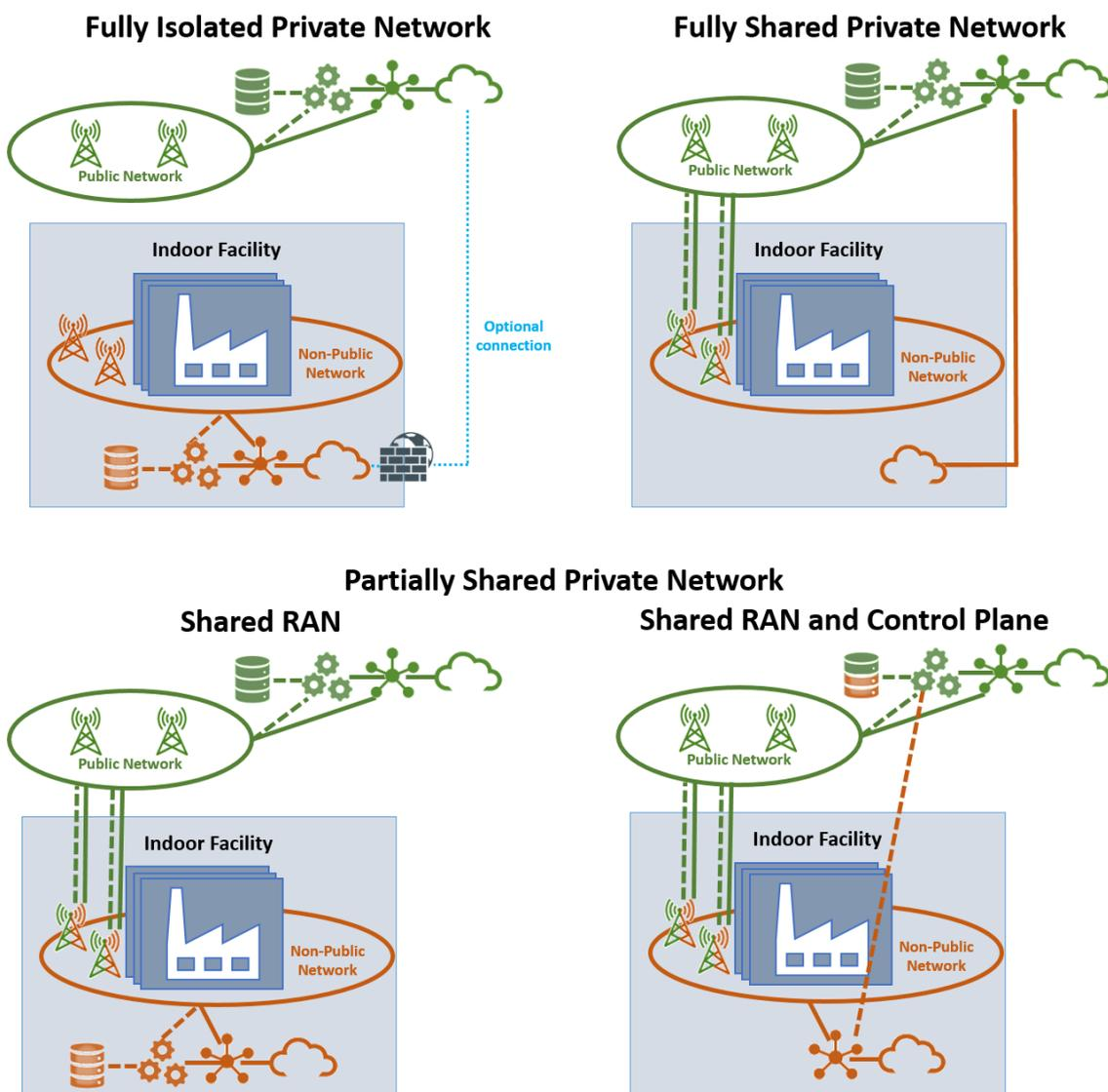
**Figure 3-28 5G NPN-PN deployment options according to 5G-ACIA**
