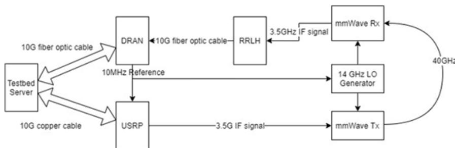
**Figure 5-65 Testbed system setup for mmWave uplink measurement**
