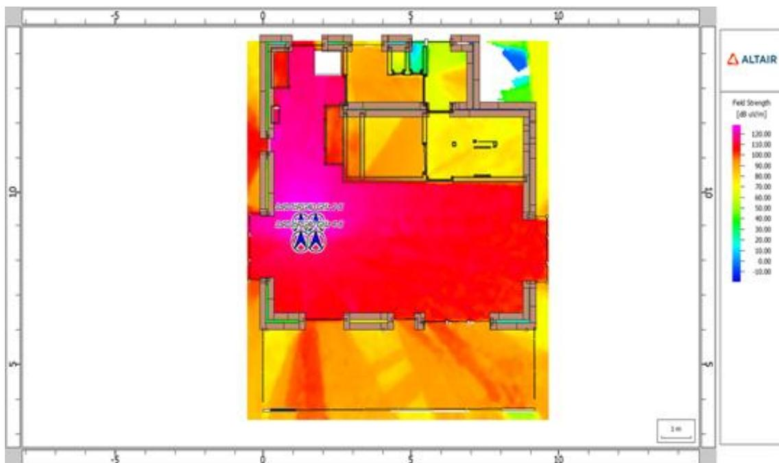
Figure 5-61 Simulation of EM radiation in integer house upper ground floor
