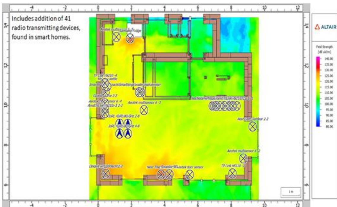
Figure 5-62 Measurement of EM radiation in integer house upper Ground floor – addition of multiple sources of radiation
