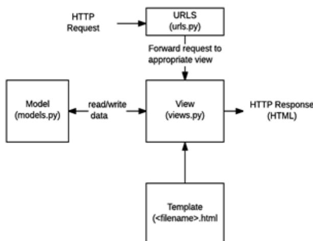
**Figure 2-15 Front-end of dynamically extensible location database**
