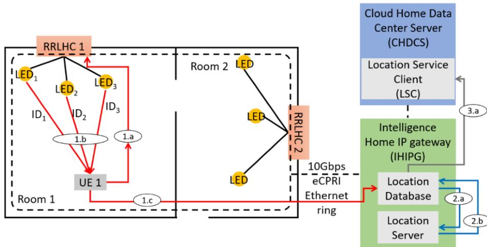
Figure 4-44 Indoor 5G visible light positioning protocol
