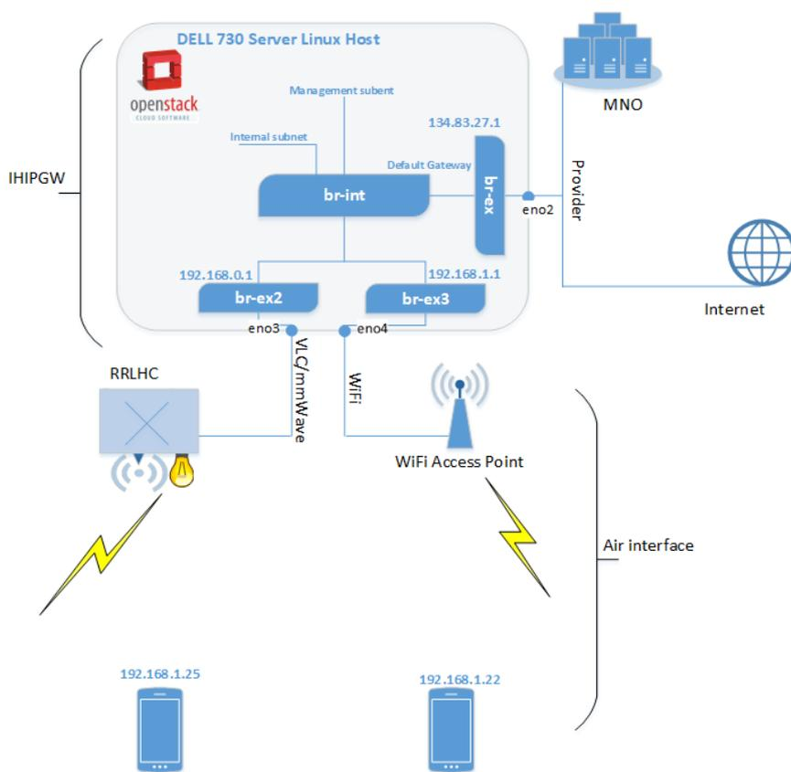
Figure 4-42 Illustration of the network architecture including MEC cloud
