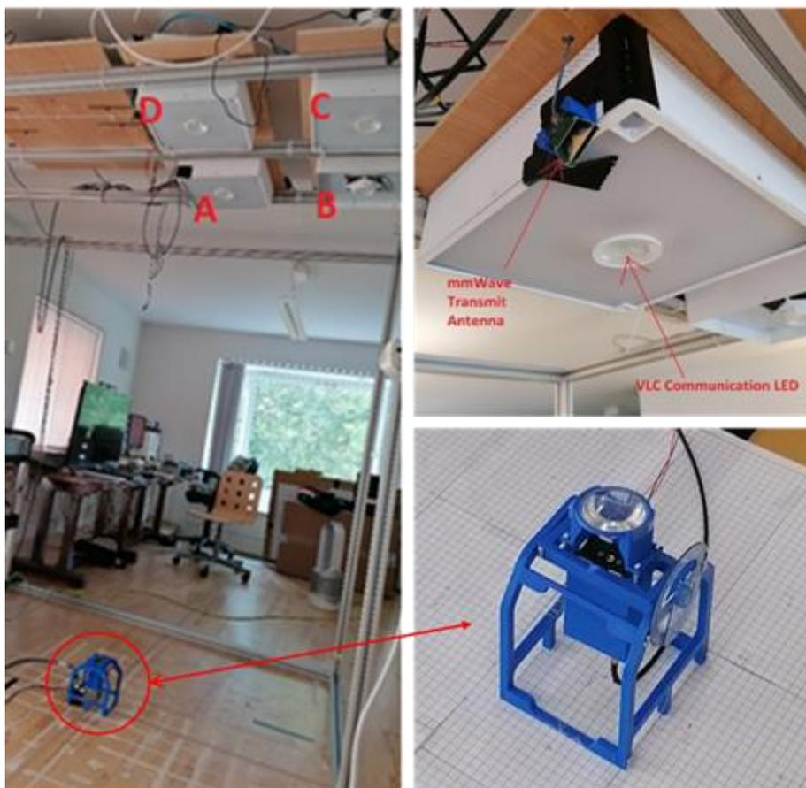
**Figure 5-67 LEDs and APD receiver with lens**
