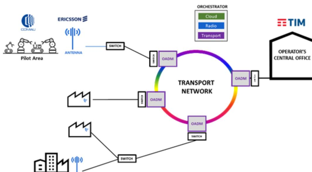
**Figure 4-41 Example configuration for shared transport network for connecting NPN**
