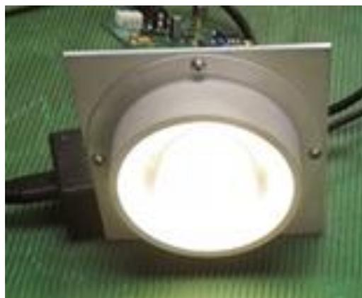
**Figure 3-21 Communication LED with circular aperture lens**
