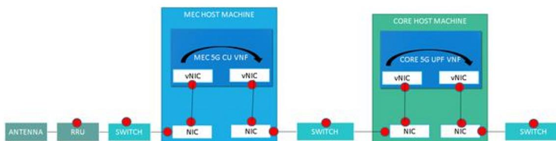
**Figure 4-52 Hardware-based data plane network slicing**
