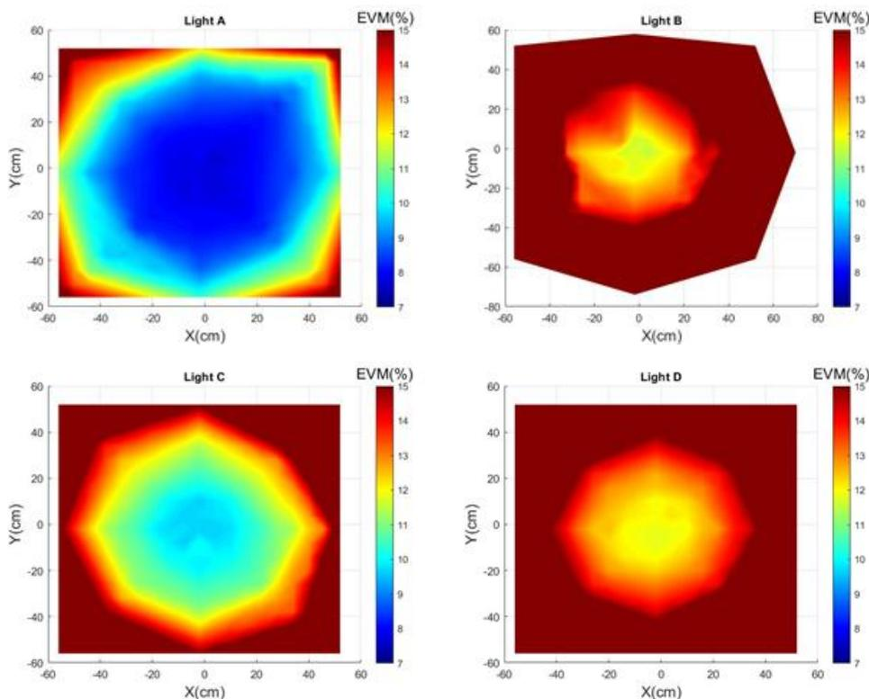
**Figure 5-64 4 VLC LED TXs EVM test Rx at ground level pointing towards communication LED and illumination LEDs off**
