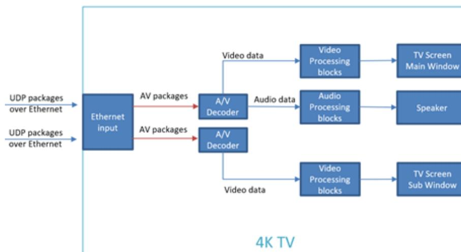
Figure 6-73 Basic diagram of Android based 4K TV application
