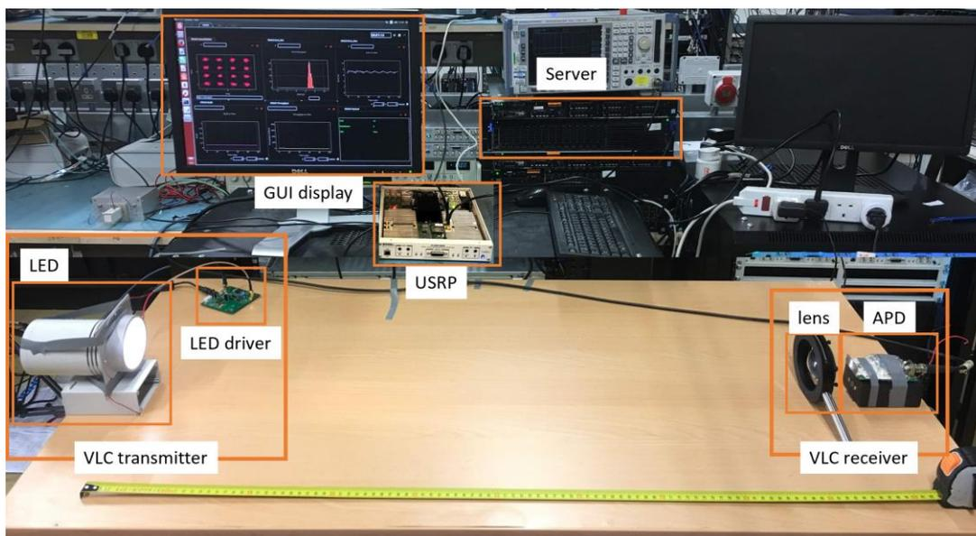
Figure 4-35 Experimentation environment of the VLC transmitter-receiver
