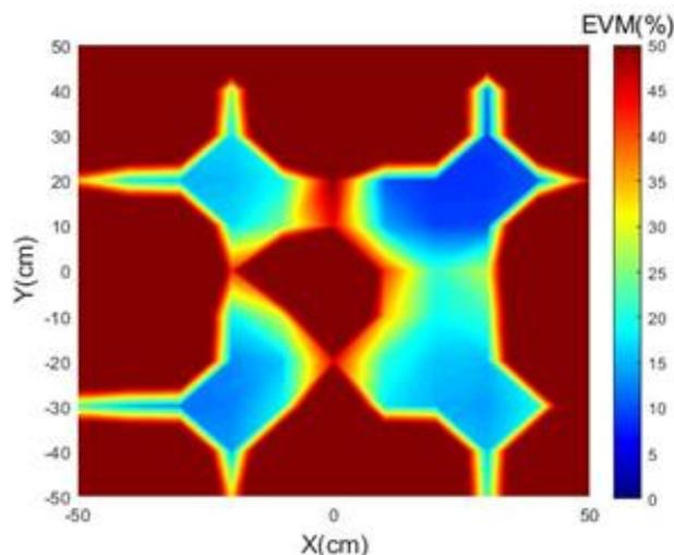
**Figure 5-63 4 VLC LED TXs EVM test Rx at ground level pointing vertically up LED A and illumination LEDs off – top Right, B – bottom right, C – bottom left, D – top left**
