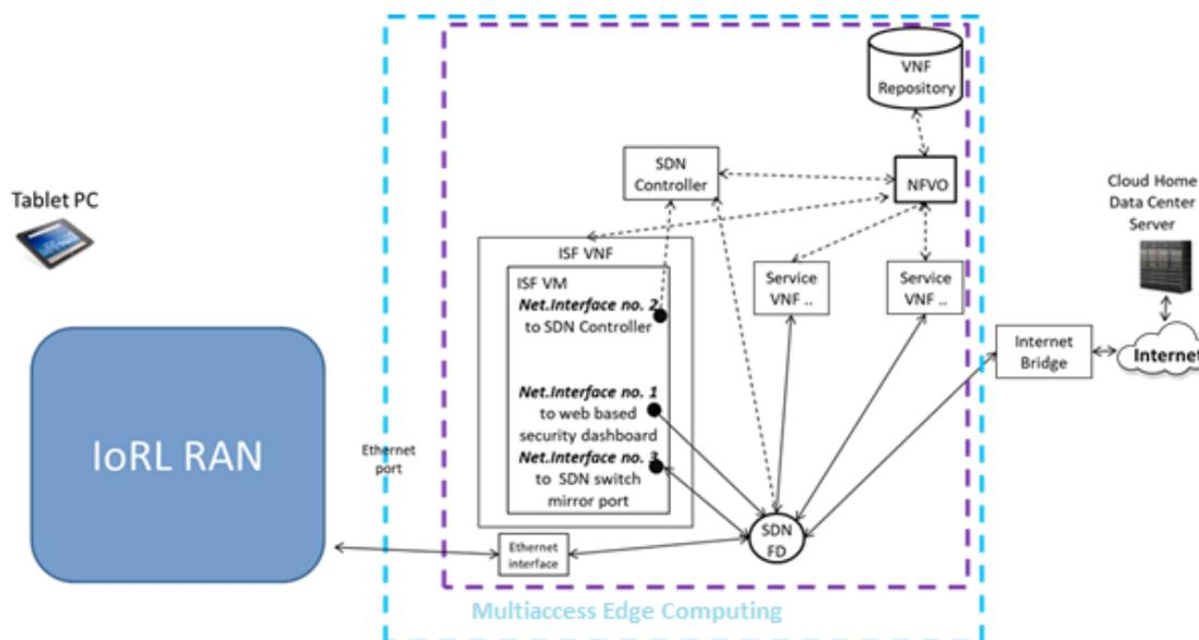
Figure 4-47 Integrated security framework in MEC
