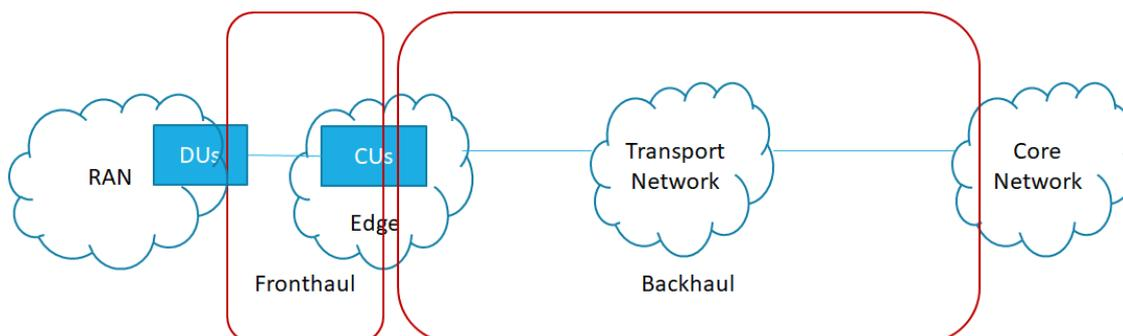
**Figure 4-51 Positioning of fronthaul and backhaul in E2E network**
