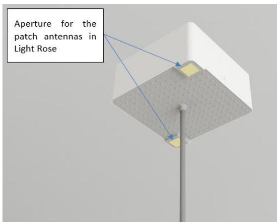
**Figure 3-24 Light rose with apertures for LED at the end of the pendant mmWave antennas**
