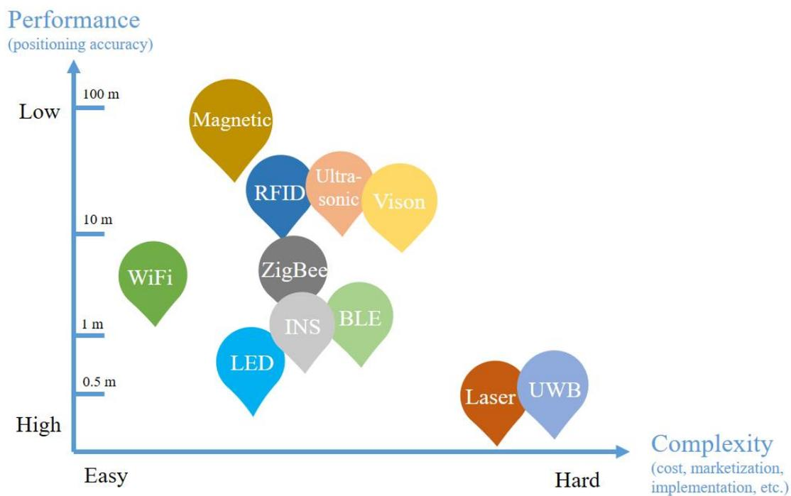
Figure 4-54 Comparison of different indoor positioning technologies
