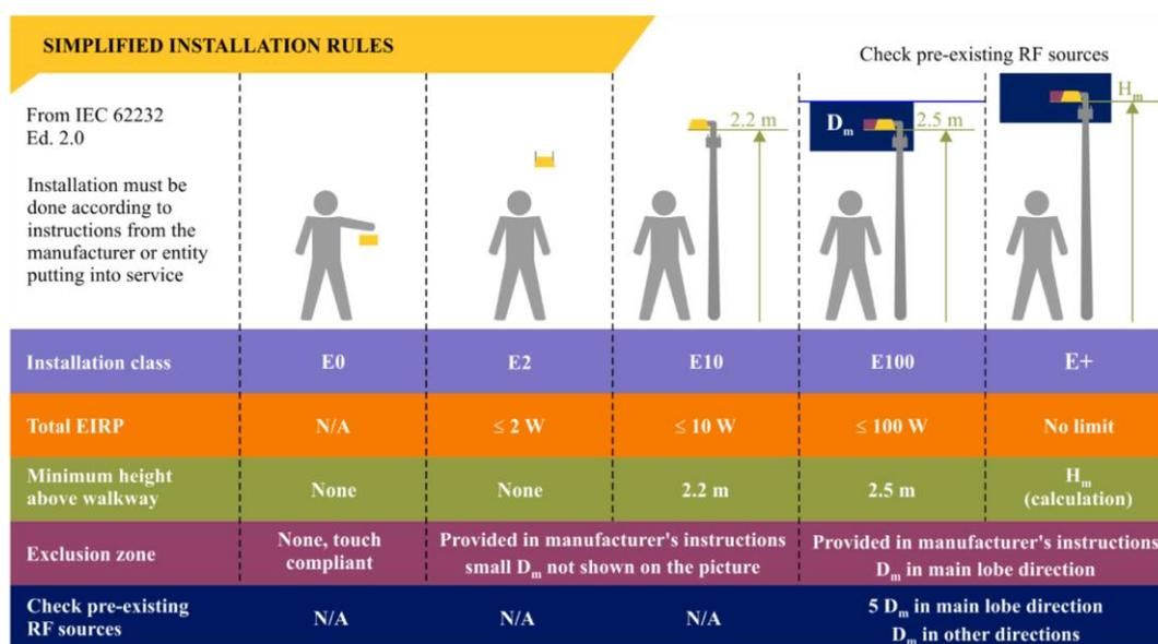
**Figure 4-39 Simplified installation rules (Source: IEC 62232 Ed.2.0 [70])**
