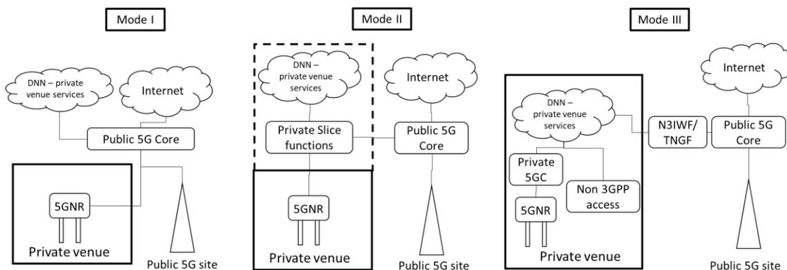
**Figure 4-40. Interconnection modes between NPN and PLMN**
