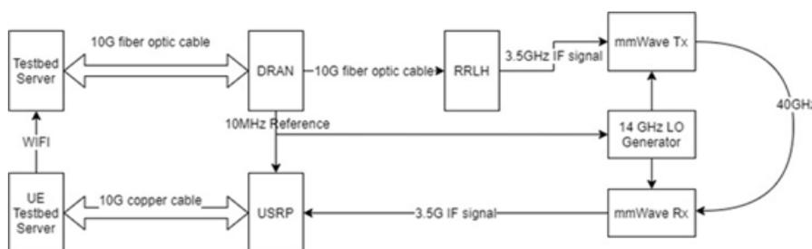
**Figure 5-66 Testbed system setup for mmWave downlink and Wi-Fi measurement**
