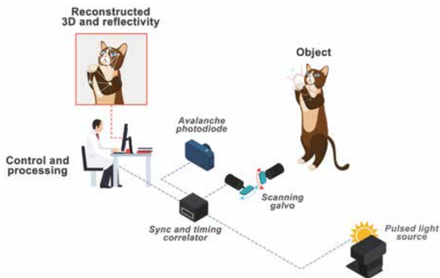
Figure 3-5 | Conceptual diagram of the quantum lidar realized by Boston University
