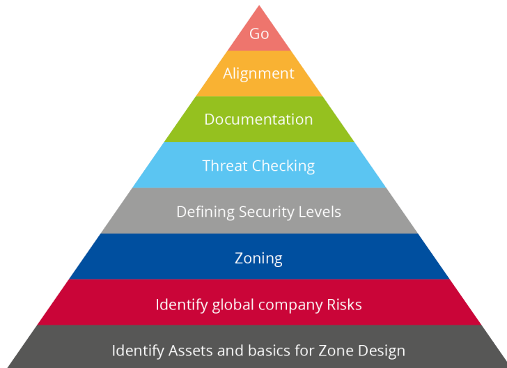
Figure 1 Zoning and conduit methodology
