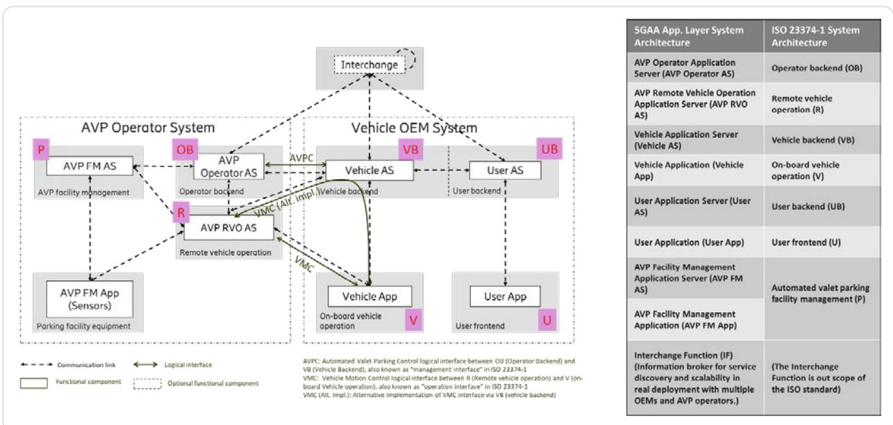
Figure 2: Application-level system architecture for AVP Type-2
