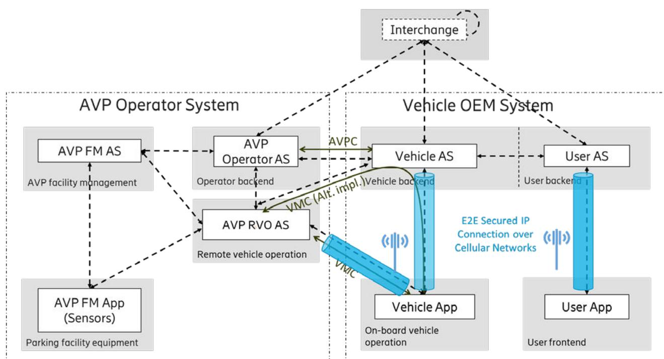
Figure 19: Architecture of cellular network-based AVP implementation
