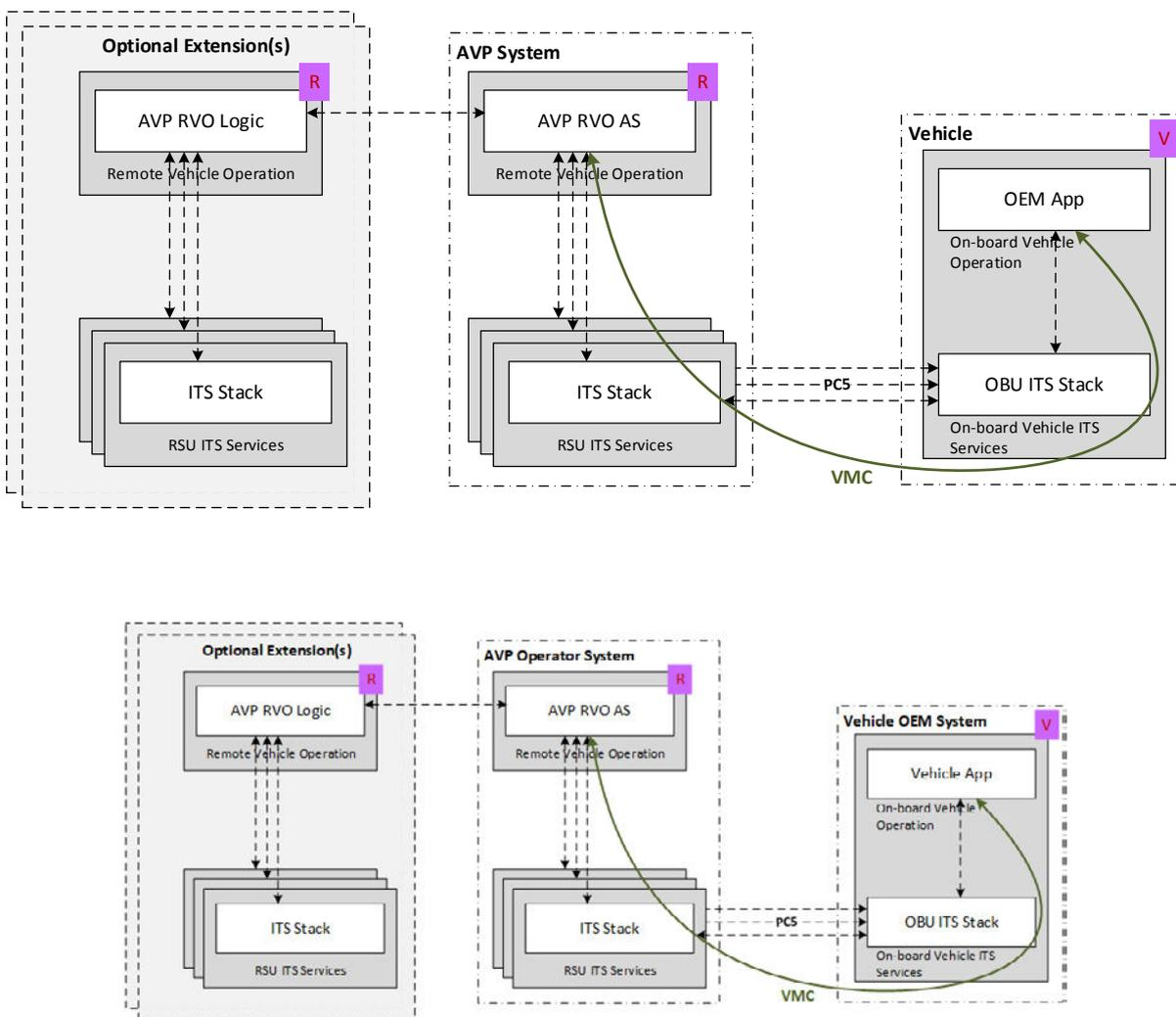
Figure 24: Split RSU/RVO architecture
