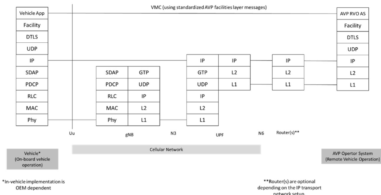
Figure 22: Example protocol stacks for vehicle motion control
