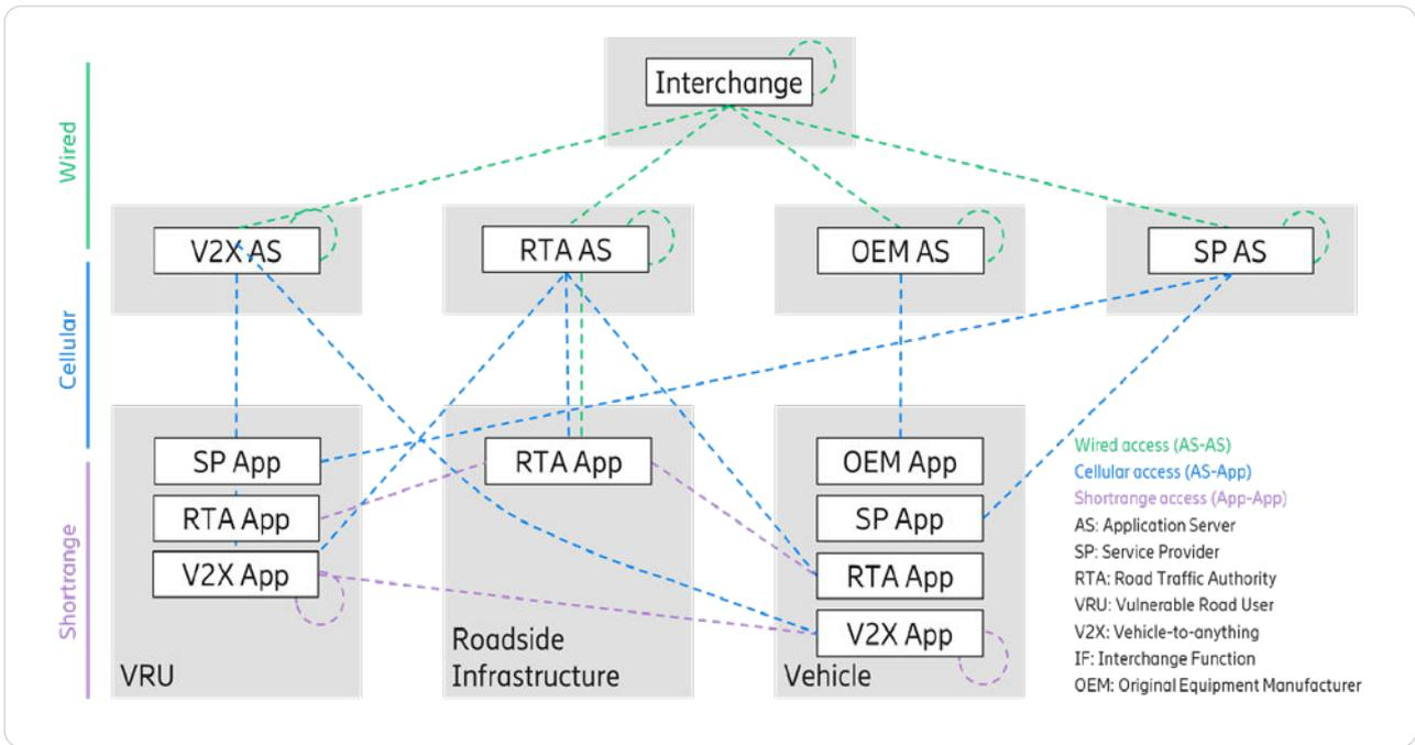
Figure 1: 5GAA V2X application layer reference architecture [2]
