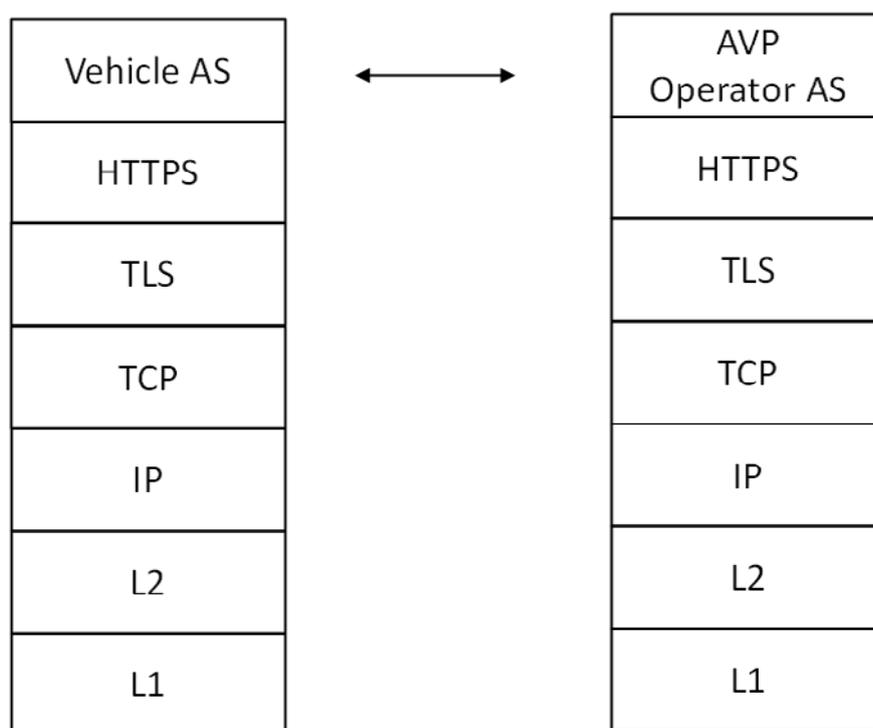
*Figure 21: Example protocol stacks for Vehicle AS and AVP Operator AS interaction*
