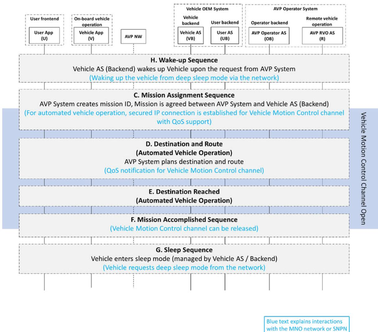
Figure 6: High-level communication sequences for AVP Type-2 re-park process
